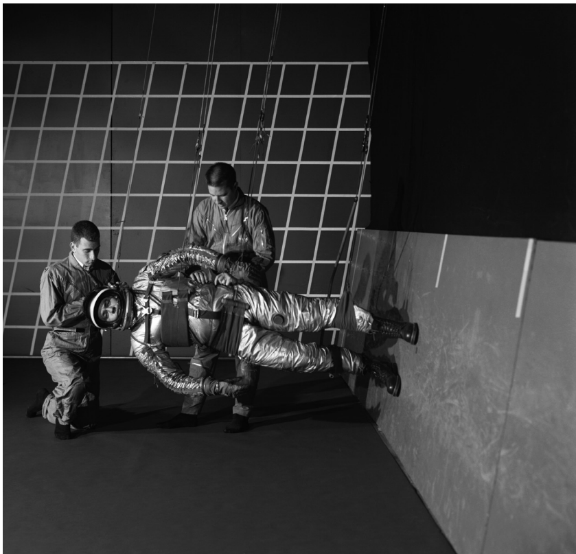
A test subject being suited up for studies on the “Reduced Gravity Walking Simulator” in the hangar at Langley Research Center, NASA 1963.
