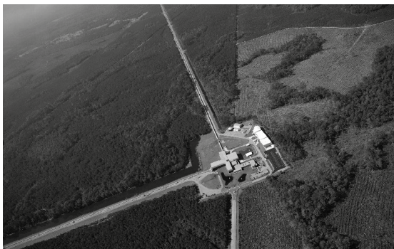
The LIGO (Laser Interferometer Gravitational-Wave Observatory) is a 4 km long observatory to detect cosmic gravitational waves and to develop gravitational-wave observations as an astronomical tool, located in Hanford, US.
